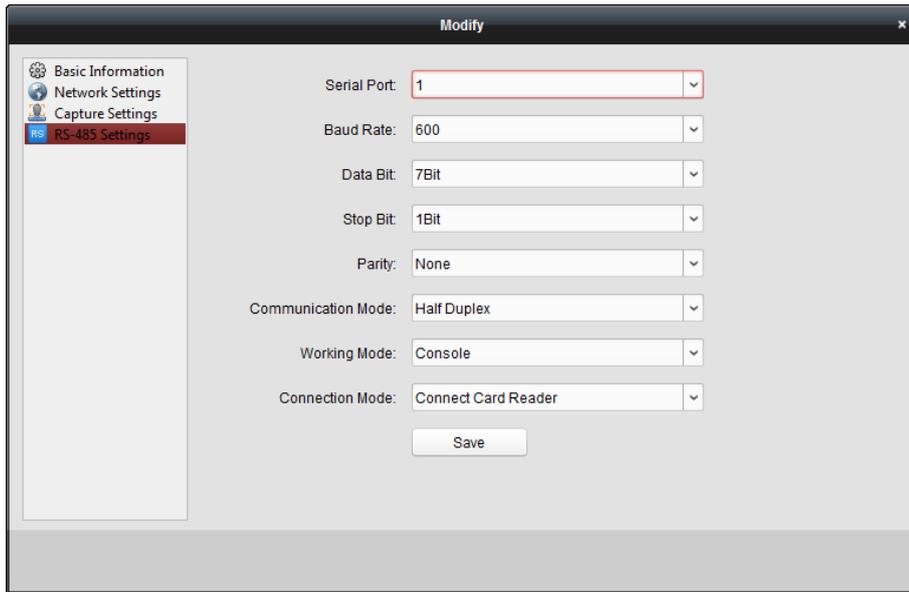
2. Select the serial No. of the port from the dropdown list to set the RS-485 parameters.
