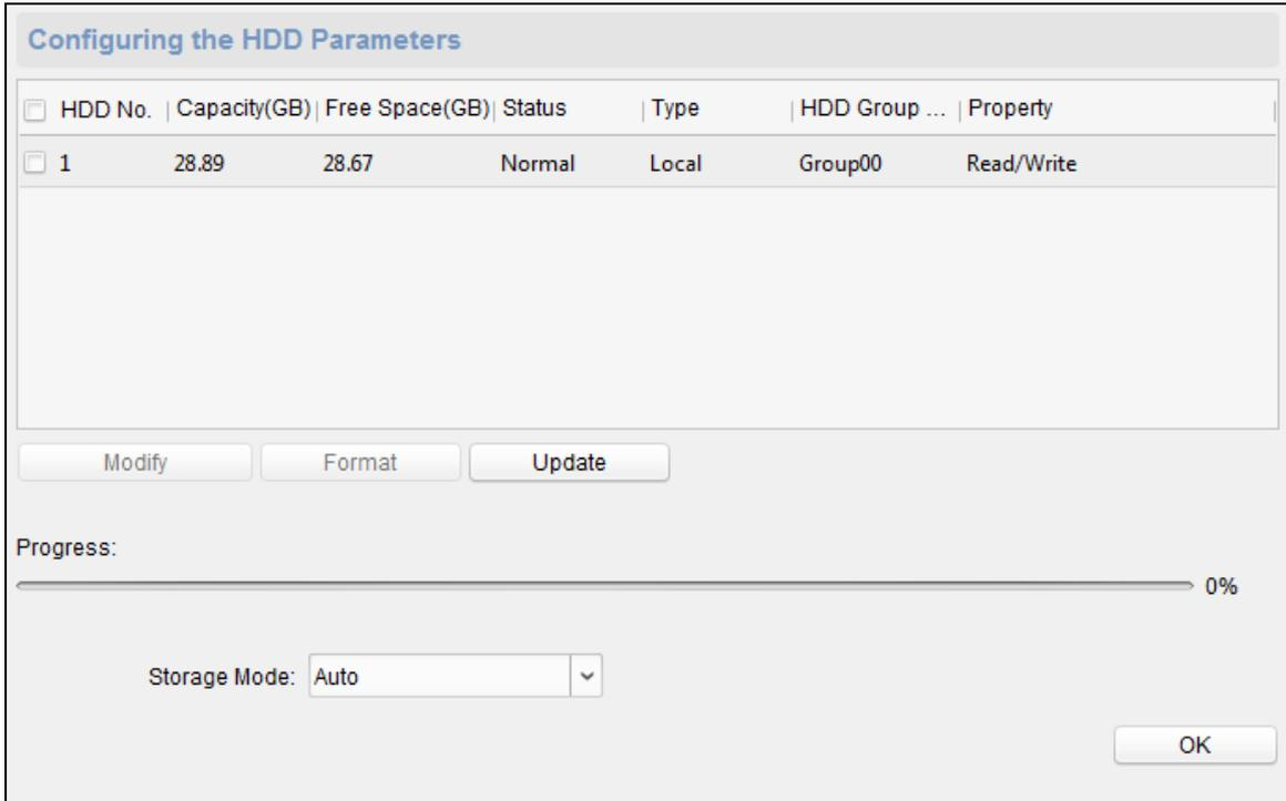
2. Check the HDD (SD card) No., capacity, the free space, the status and so on. You can also edit and format the HDD (SD card). Or click **Update** to refresh the data.
