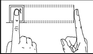
You should press your finger on the scanner horizontally. The center of your scanned finger should align with the scanner center.
